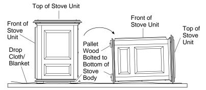
Figure 7 - Laying Down Stove On Side
